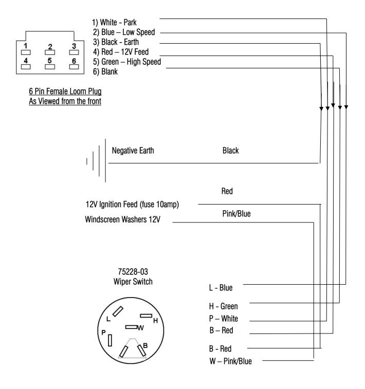
Wiper switch system is 12V Positive Feed
