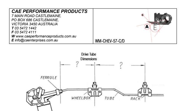
To have centred parking, as was on the original 1957 Chev, the L.H. side (passengers) wheel box is fitted with Bundy tubing running to the top of the wheel box. I.E. The wheel box is fitted upside down I.E turned 180 degrees. The R.H. Wheelbox has the tubing and drive cable running on the bottom of the wheelbox gear. i.e 180 degrees to the position of the L.H. side. For L.H.Drive vehicles the wheelboxes and wiper motor mounting is completely opposite to the above instructions.
